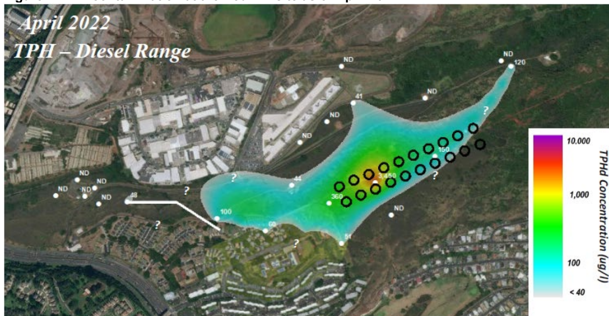
Figure 4: TPH contamination at the Red Hill site as of April 2022
